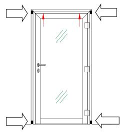
2. Align and wedge the frame into the opening, using temporary packers at the corners.
