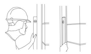
**3.** Ensure that the frame is vertical in both planes, particularly the hinge jamb, and that the door head is still parallel to the frame head.
