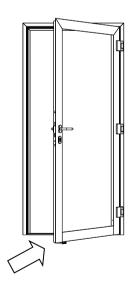
**4.** Open the door carefully to approx. 45°, taking care not to disturb the frame, then temporarily pack the lock edge of the door leaf off the floor, keeping the hinge jamb vertical.
