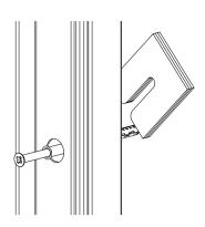
**5b.** The frame fixings need to pass through permanent packers. This is best achieved by loosely securing each frame fixing into the wall, then hammering packers into position on the fixing, before fully tightening the fixing.
